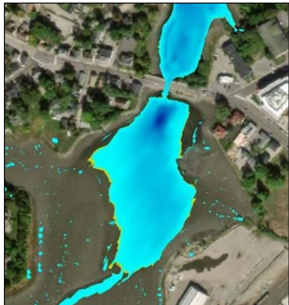
Figure 17 – Inundated areas at the MLLW tide stage trough with blue shading representing the post-project inundation area and yellow shading indicating the additional areas inundated under pre-project conditions
